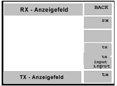
After pressing the appropriate key, the field lights up yellow for ca. 3 seconds. During this time, DiSEqC commands can be received and assessed. The display of the received DiSEqC command appears in the RC display field.
